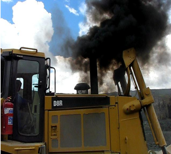
Figure 1: Optical presentation of Phase 2 of the fuel enhancement evaluation at Letšeng Diamond Mine before addition of product C.
