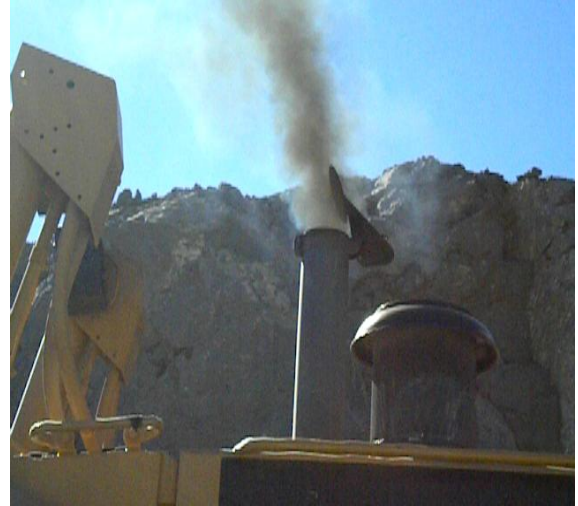
Figure 2: Optical presentation of the reduction in smoke 21 days after addition of product C during the fuel enhancement project at Letšeng Diamond Mine.
